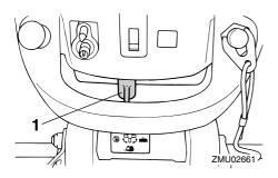
1. "OPEN" position for the built-in tank
